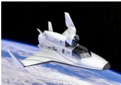
Artist's conception of the Lynx Mark III suborbital vehicle with dorsal pod payload.
