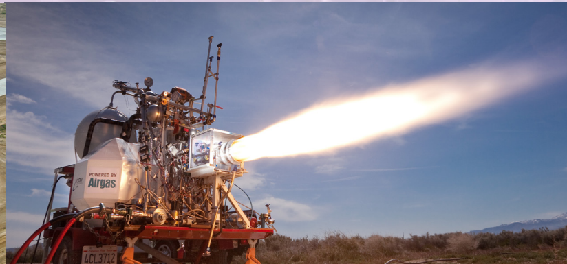
October 2012: Test firing of XCOR Aerospace's liquid oxygen/kerosene engine destined to power the company's Lynx suborbital reusable vehicle.
