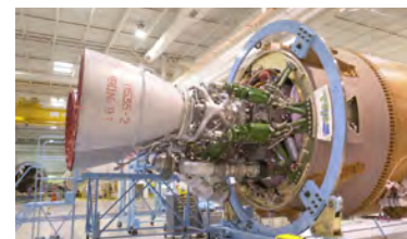
An RD-180 engine installed on the first stage of an Atlas V (ULA)
