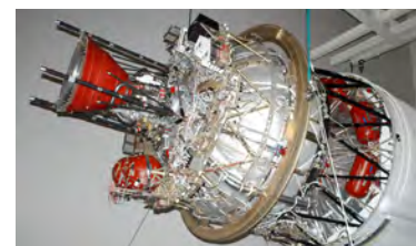
An RL10B-2 powers the Delta IV cryogenic upper stage (ULA)
