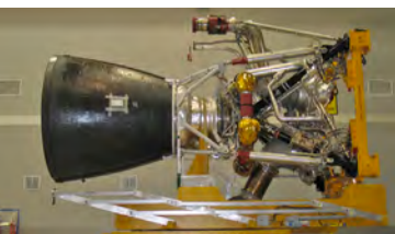
An RS-68A being prepared for installation on a Delta IV CBC (ULA)
