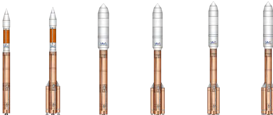
Atlas V 401/402 411/412 Atlas V 421/431 Atlas V 501/502 511/512 Atlas V 521/522 531/532 Atlas V 541/542 Atlas V 551/552
