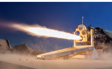
The XR-5K18 being test fired (XCOR Aerospace)
