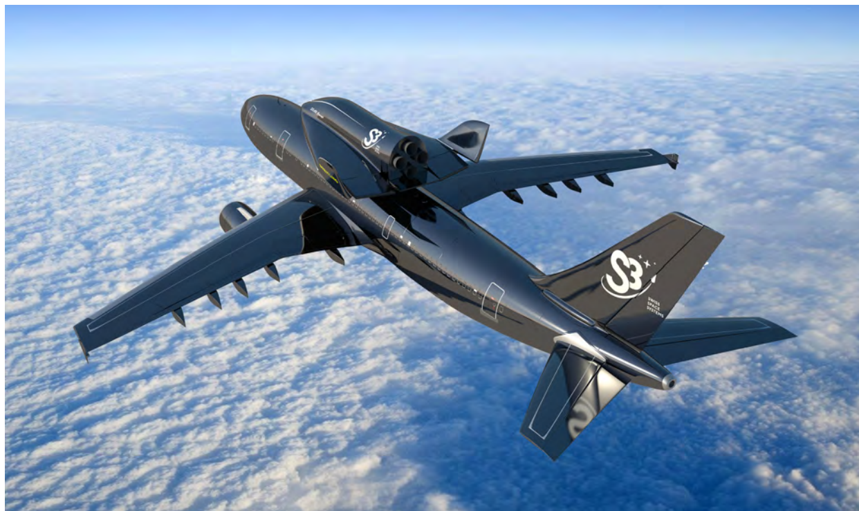
An artist's impression of SOAR and its Airbus A300 carrier aircraft in flight. Source: Swiss Space Systems
