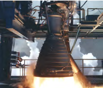
An RS-27A undergoing ground testing (ULA)
