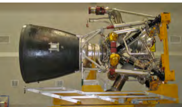
An RS-68A being prepared for installation on a Delta IV CBC (ULA)
