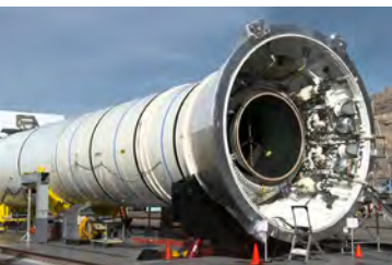
A 5-segment Solid Rocket Booster being prepared for ground test firing (Orbital ATK)
