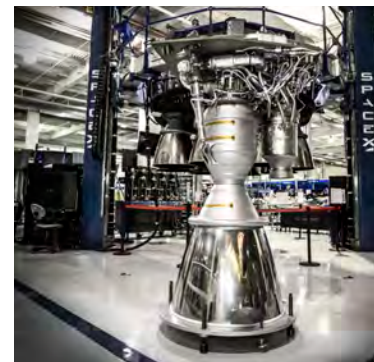
A Merlin-1D engine (SpaceX)
