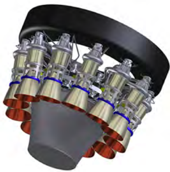
The FRE-2 aerospike engine (Firefly Space Systems)
