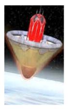
Fifteen seconds after apogee is reached a reentry ballute is deployed and a high temperature cone around the base area is inflated. (This cone is later used as the landing absorption cushion to protect the engines.) The ballute is used to increase surface area and maintain passive static stability of the reentering capsule. The main parachute deploys
