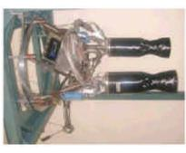
used on da Vinci, burning kerosene with liquid oxygen in a helium pressure fed system to generate 10,000 pounds of thrust. The rocket engines, the entire propulsion subsystem, and the flight guidance system are being supplied by the DVP propulsion team in California, USA. Ground firing and flight testing have occurred already.
