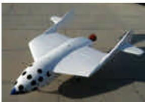
SpaceShipOne (SS1) is a three-place, high-altitude research rocket, designed for sub-orbital flights to 100 km altitude. The unique configuration
