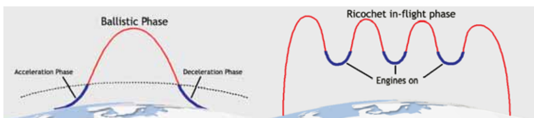
Figure 2-3: Ballistic and Ricochet flight profiles
