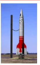
The Canadian Arrow is a 54-ft long, two-stage, three person sub-orbital rocket with the second stage doubling as an escape system. The first stage is 33.5 ft. long and 5.4 ft. in diameter with four fins at the base for aerodynamic stability.
