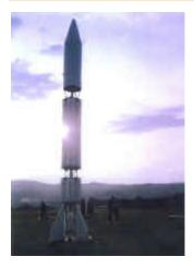
The Orizont vehicle is extremely simple to ensure a high reliability and low production cost. The entire vehicle has a length of 14 meters, a diameter of 1.3 meters, and weighs 7,000 kg (15,430 lb<sub>m</sub>).
