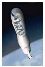
The Advent spacecraft is launched vertically from water and landed horizontally like a sea plane. It is a winged rocket that is designed to glide down to the ocean surface for a safe, controlled landing.
